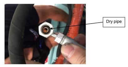
Analysis revealed that this obstruction is due to a solder run which occurred during soldering of the lower union of the pipe, thus making the oil flow impossible.
