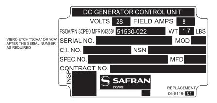
NOTE: THE SERIAL NO. AND MANUFACTURE DATE (MFD) MUST BE TRANSFERRED FROM OLD ID. PLATE.
